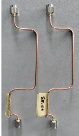
Semi-rigid cable assembly with different types of bends
